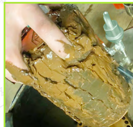
Non-magnetic dirt and debris captured by the Anti-Microbial Cartridge Filter
